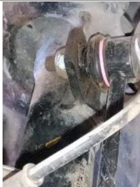
Left stabilizer link leaking g
