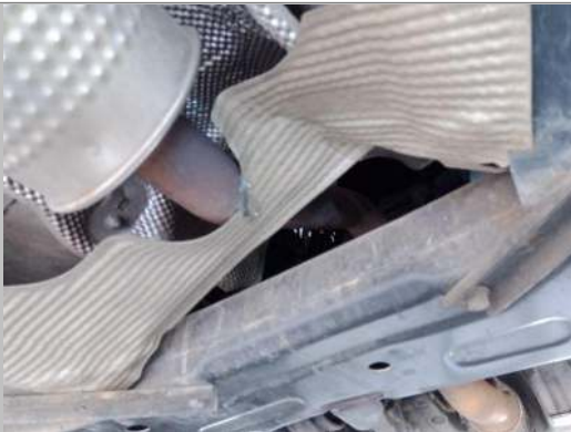
Engine to silencer pipe
