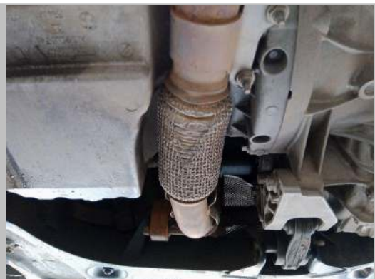
Engine to silencer pipe
