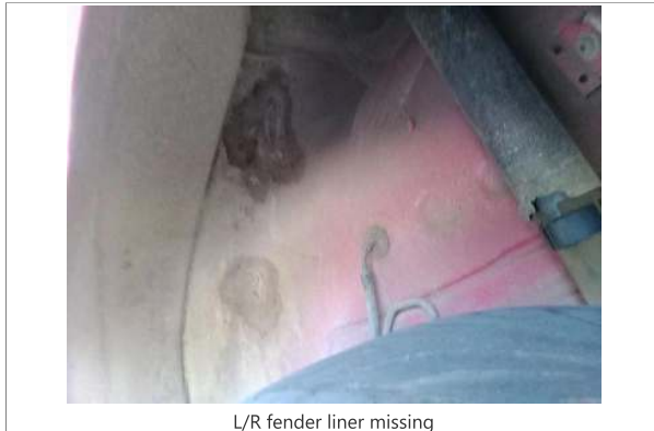
L/R fender liner missing
