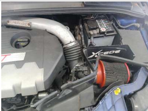
Aftermarket air filter fitted
