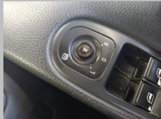
Electric mirror knob damaged
