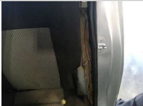
L/R inner seat panel missing
