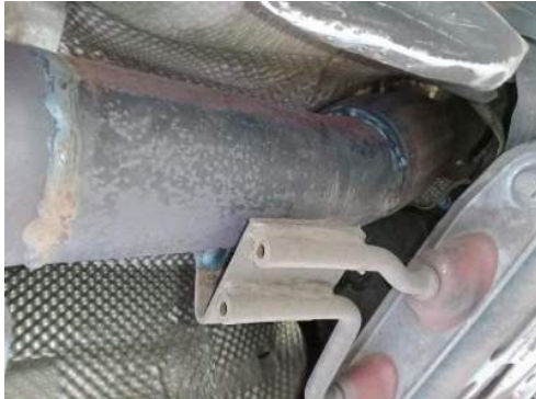
Engine to silencer pipe
