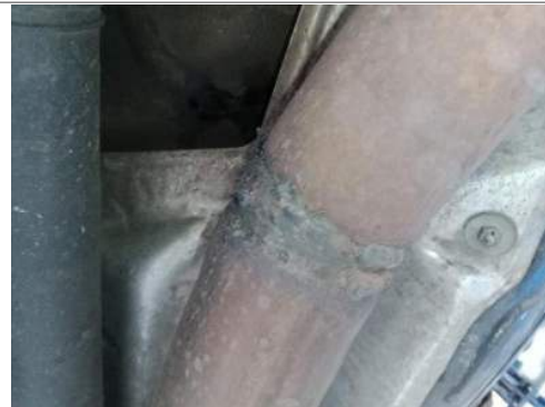
Engine to silencer pipe
