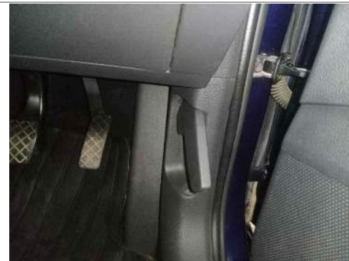
Bonnet release handle damaged
